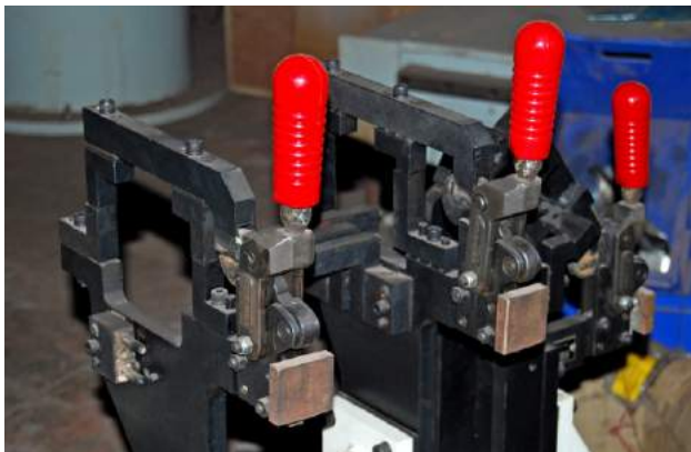
HV Series Clamp in a BIW fixture
