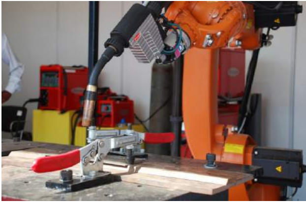
H-45105-UB on Co2 Welding fixture
