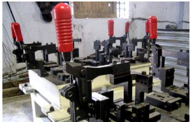
HV Series in a fixture used with standard shims
