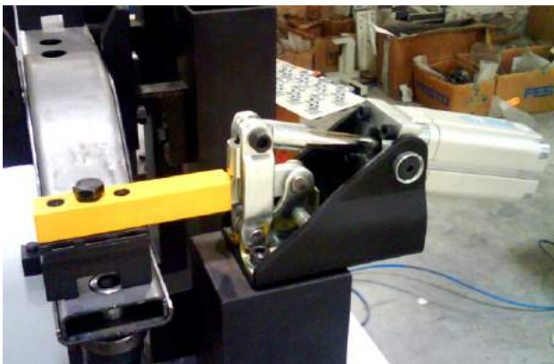
AOT-3586-SB used in a checking fixture
